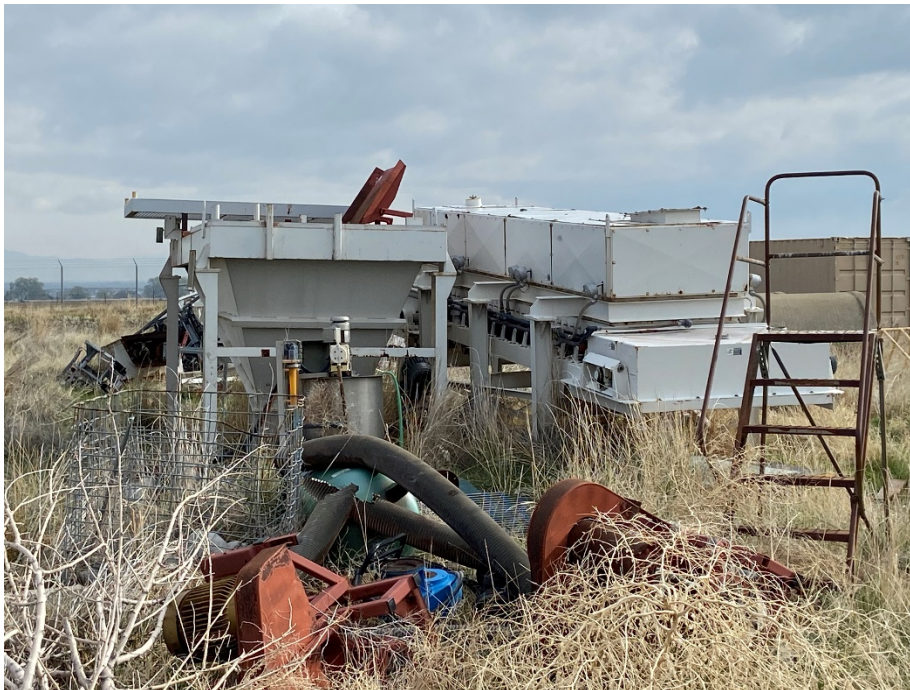
Pile #4: Sludge hopper, lime activation system, sludge handling equipment, railing, step screen, pumps (all of these items were part of the old sludge process that was scrapped out when the green house was constructed).
